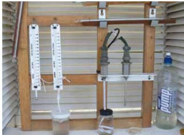
Figure 5. The internal view of a small Stevenson screen set up with both in-glass and platinum resistance probes.
