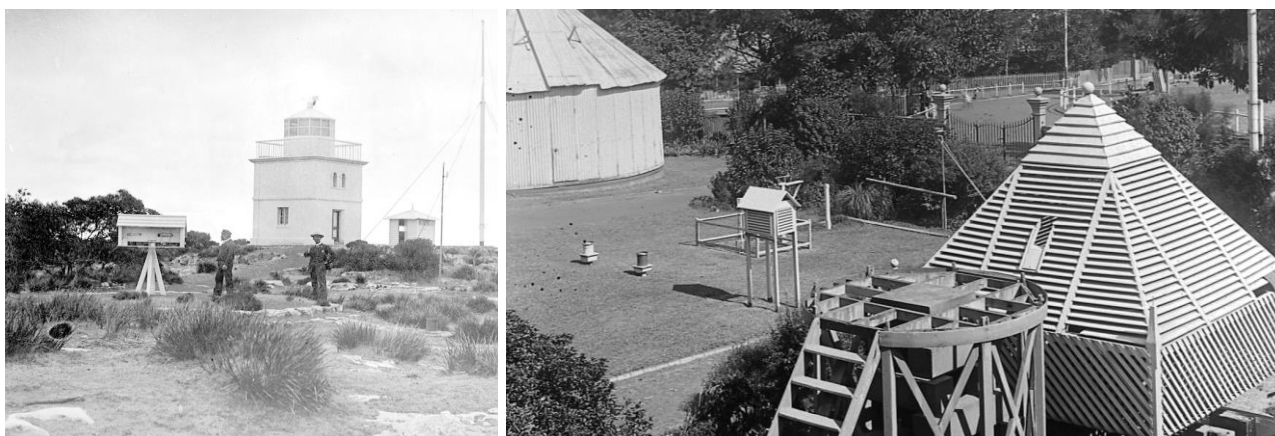
Figure 1. Temperatures measured in the open-fronted Glaisher stand at Cape Borda lightstation, Kangaroo Island SA in 1903 and the pyramid-like 'thermometer house' at Sydney Observatory before 1908 are not necessarily comparable with those measured in Stevenson screens, such as the one in the centre of the Observatory lawn. (Photographs courtesy of the State Library of South Australia (L) and the Museum of Applied Arts and sciences, Sydney (R).)
